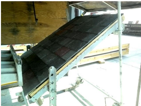
Deck #1: At End of Testing (160 mph)
