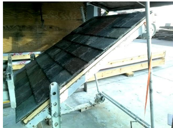
Deck #2: At End of Testing (160 mph)
