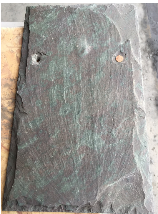
Figure 1: Traditional punching machine (left) and a machine punched, Vermont Mottled Green and Purple slate (right).
