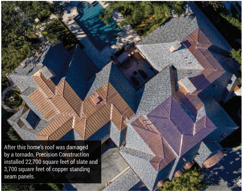
After this home's roof was damaged by a tornado, Precision Construction installed 22,700 square feet of slate and 3,700 square feet of copper standing seam panels.
