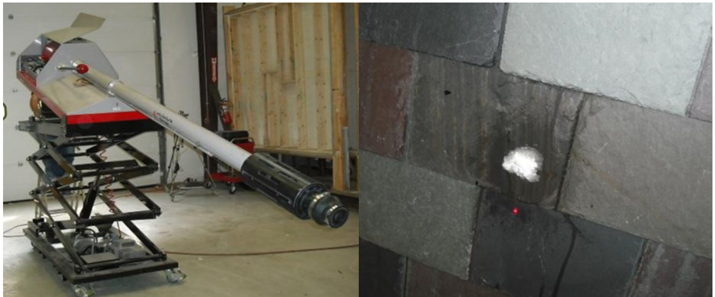
Figure 3: Ice ball cannon (left) and impact zone (right) during impact resistance testing of natural slate shingles in accordance with FM 4473.
