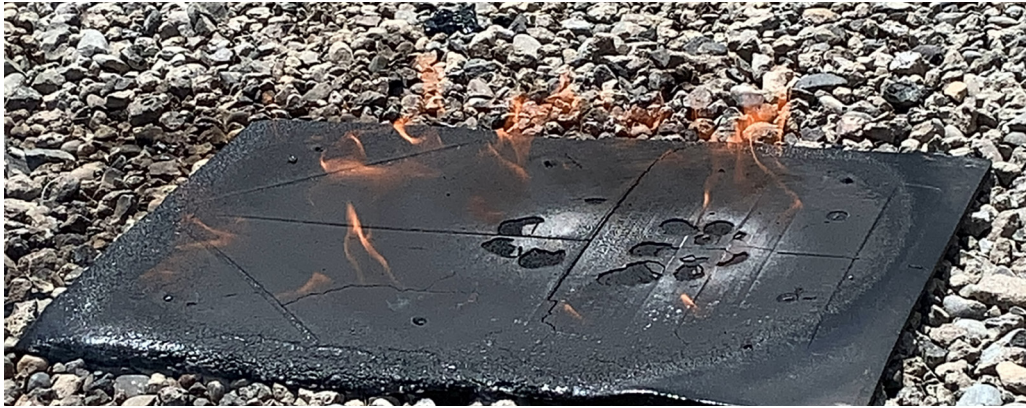
Figure 2: Burning and charred synthetic shingle.
