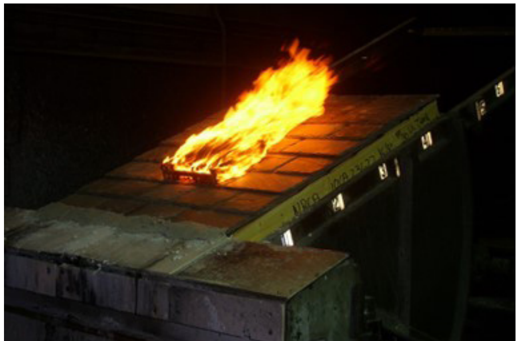
Figure 1: Slate roof assembly undergoing the burning brand test in accordance with UL 790, Standard Test Methods for Fire Tests of Roof Coverings.
